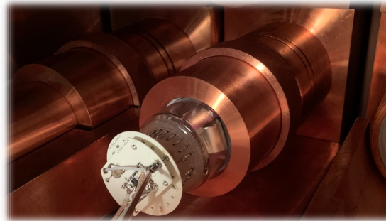
Voltage divider + preamp on Pyralux support
